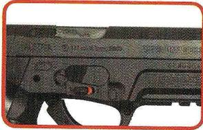
**7** Push the Safety downwards to the "Off Safe" position. The Airgun is now ready to fire. Pull the trigger to shoot with the Airgun. After firing, return the safety to the "On Safe" position.
